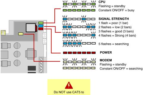
power this device as damage will occur. 0-6ft - 0.5mm<sup>2</sup> (20 gauge) 6-12ft - 0.75mm<sup>2</sup> (18 gauge) 12-24ft - 1mm<sup>2</sup> (16 gauge)
